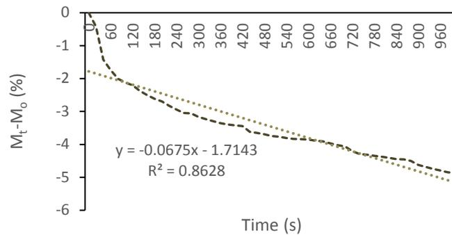
Fig. 8. Plot of  $M_t - M_o$  vs  $t$  of microwave drying of oil-palm shell at 60 °C.
