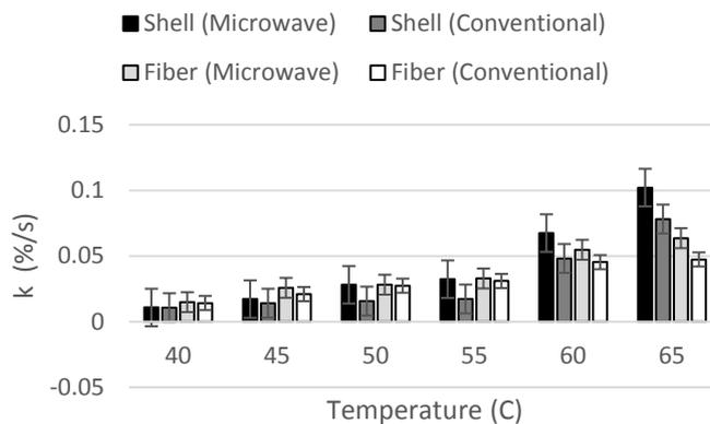
Fig. 9. Drying rate constant during constant period.
