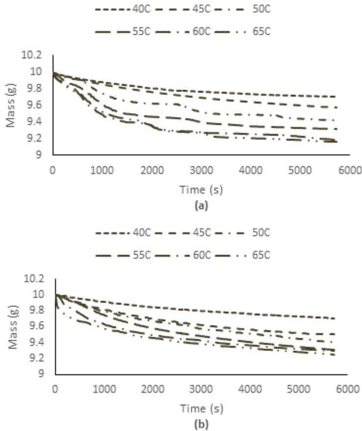
**Fig. 4. Drying curves of palm oil fiber: (a) conventional, (b) microwave.**
