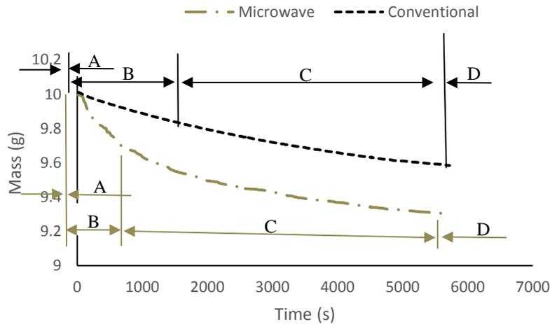
**Fig. 5. Drying process of oil-palm shell using microwave and conventional oven at 60 °C.**
