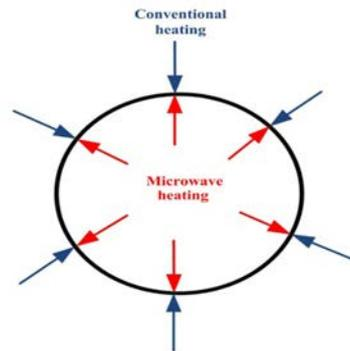
**Fig. 2. The difference in the heating process using conventional heating and microwave [23].**
