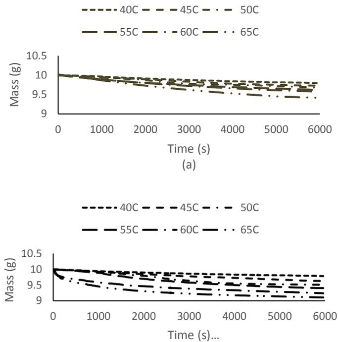
**Fig. 3. Drying curves of palm oil shell: (a) conventional, and (b) microwave.**
