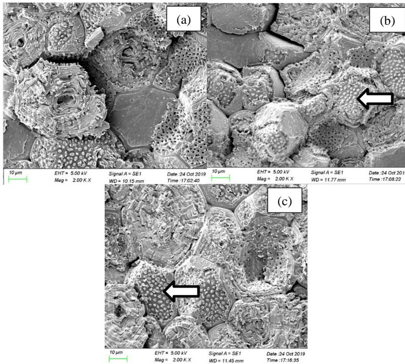
**Fig. 12. Surface morphology structure of oil-palm shell (2000x):**
