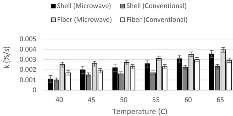
Fig. 10. Drying rate constant during falling rate period.
