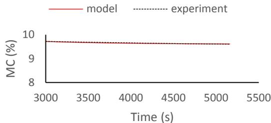
**Fig. 6. Experimental and simulated curves for the falling rate period conventional drying of oil-palm shell at 60 °C.**
