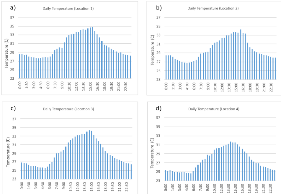
Fig. 6. Graph of a daily air temperature of sample points: (a) settlements 1, (b) industrial buildings, (c) settlements 2, and (d) rice fields on December 13, 2021
